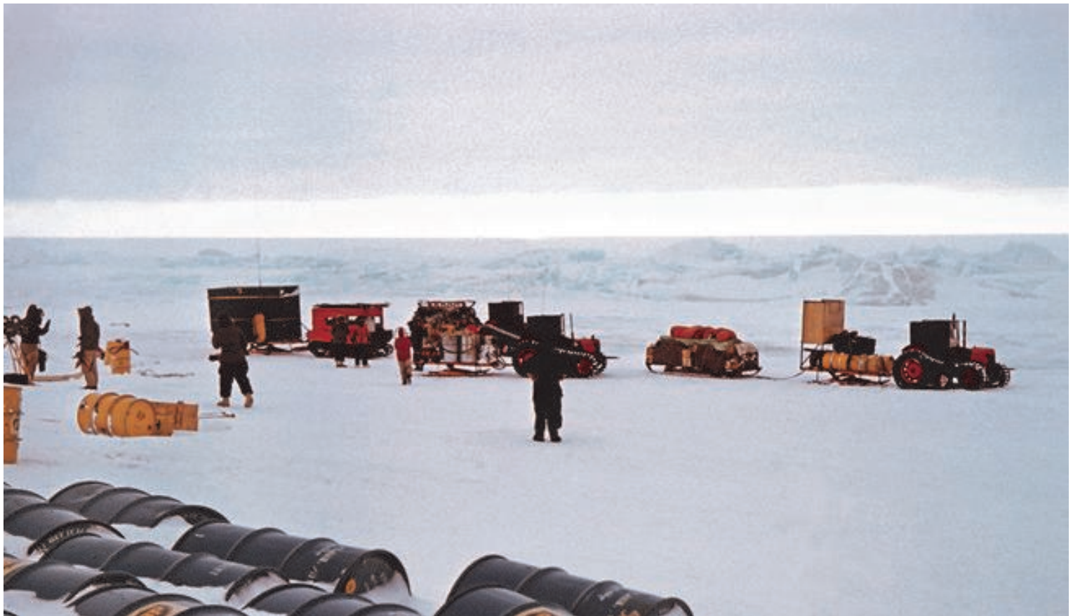
Hillary's tractor party getting ready their polar trip. Behind the first Ferguson tractor is the "crows nest" that they built for better visibility when traveling. It was soon discarded as the visibility was no better than when standing while driving the tractor. The Weasel is in the rear pulling the caboose. Photo credit: Geoffrey Lee Martin
