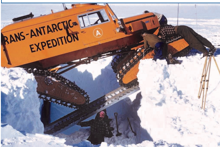
Sno-Cat Able fell into a 25 foot crevasse. The crevasse was filled partially with snow so they could stand under able and install the 14 foot long crevasse bridging. It took two Sno-Cats to pull Able out.
