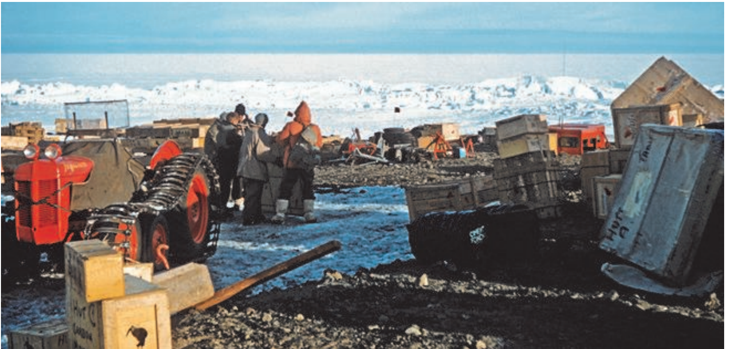
Unloading supplies at Scott Base. The first tracks had chain links that wore out fast with the rock grit at the base. Notice the red cab of the Weasel in the back ground. It was removed incase the vehicle fell through the ice and those inside had to make a fast escape. Photo credit Geoffrey Lee Martin
