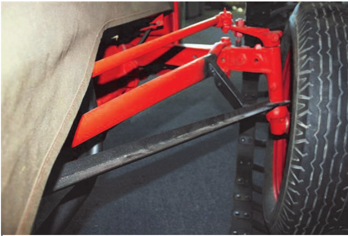
The black pieces are the pieces of Waratah fencing post that were used to strengthen the front axles. Photographer Belinda Weir, credit Sir Edmund Hillary Alpine Centre
