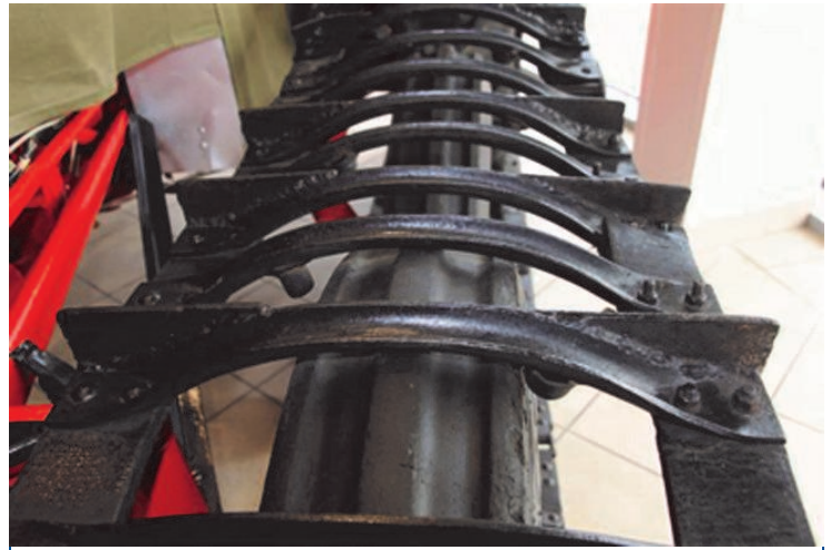
Photo of original track on "Sue" showing the extra lower lugs welded under the cleats to stop slipping around the rear tire treads, and angled steel cleats welded to every second track for extra gripping in the soft snow. The three rib tire was not the original style used in the TAE. Photo credit: John Kennedy of the UK
