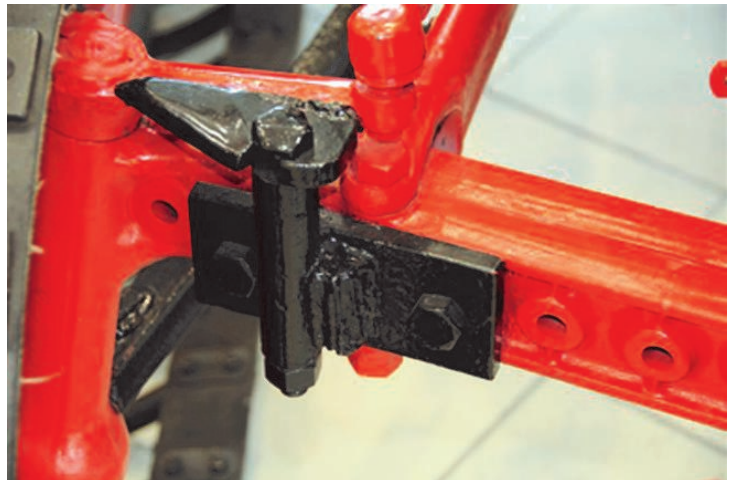
The area in black was the piece that was welded on to keep the front wheels from turning, but the front wheels were not aligned correctly. To adjust this a deeper notch was cut in the plate on top of the spindle arm. This allowed the front wheels to run true. The A frame tow bar has been cut off by a gas torch as it was no longer needed by the time the tractors left the South Pole. Photo credit Sir Edmund Hillary Alpine Center
