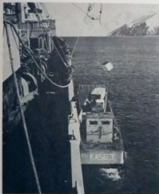
The volcanic beaches of Cape Hallett require the use of LCM landing craft for cargo operations. The LCM comes alongside and is loaded with cargo.
