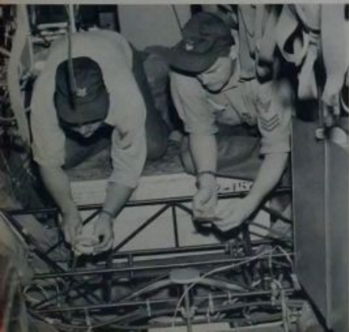
Left: A trimetrogon aerial camera mount in a P2V is worked on by Woods and Reimer before the cameras are installed.
