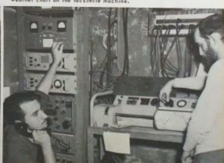
James B. Walker, RM2, talks to Christchurch over single side band while James A. Howell, TERM1, prepares to transmit a weather chart on the facsimile machine.
