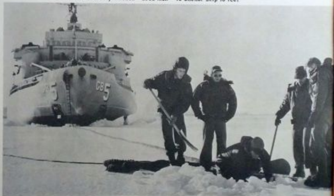
Staten Island men bury wooden "dead man" to anchor ship to ice.
