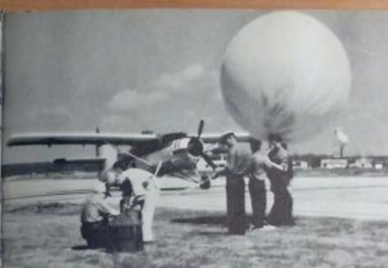
Ground handlers prepare to launch a balloon for a skyhook aerial retriever test at Quonset. Neptune retrieving gear snags the line. In real use end of line holds 2 harnesses to pick up a man.
