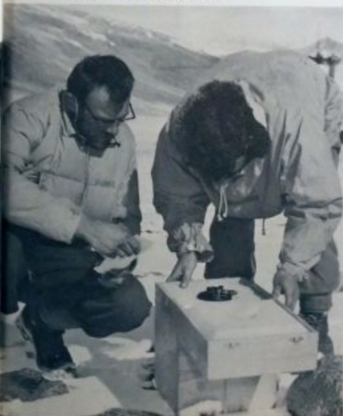
Drs. Dick Blank and Colin Bull of Victoria University, Wellington, setting up gravimeter.
