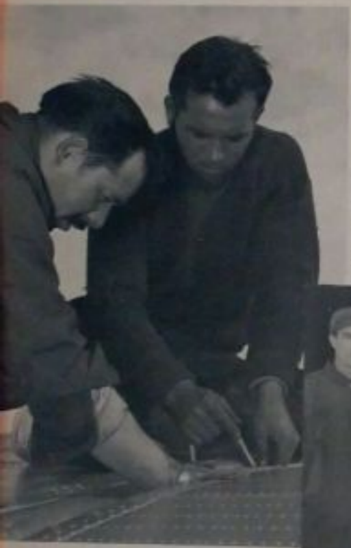
Vernon M. Leslie, AD2, and Joseph H. Latshaw, AMS2, connect electrical connections on the starboard wing before permanently affixing it to the fuselage of an Otter.
