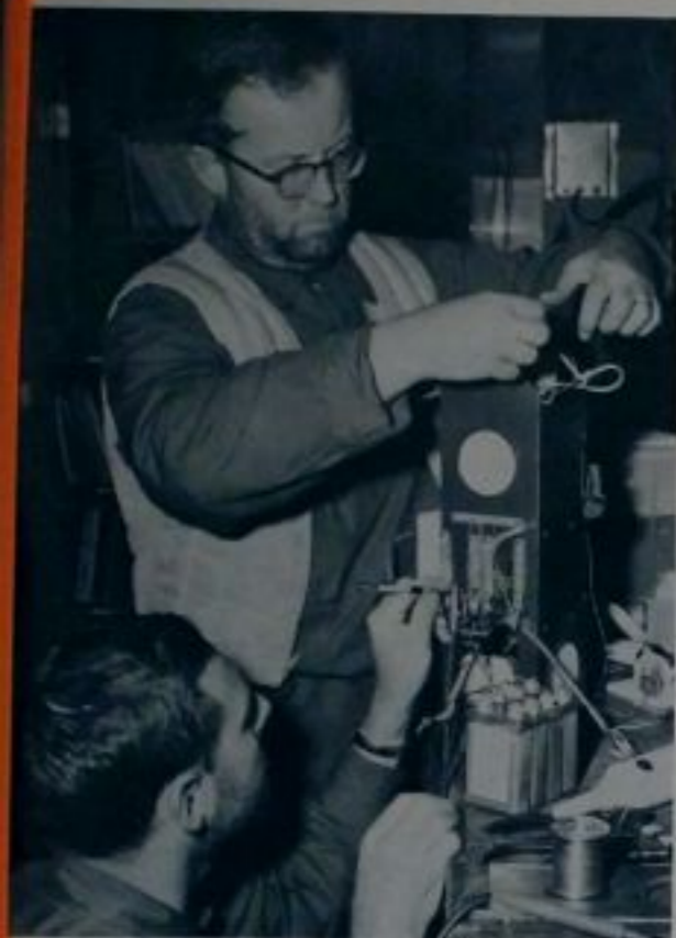
John A. Brown and Emmett J. Pybus prepare high altitude dew point hygrometer for balloon launching.
