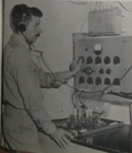
Richard H. Evans, hydrographic office, tests salinity - measuring apparatus aboard Staten Island.
