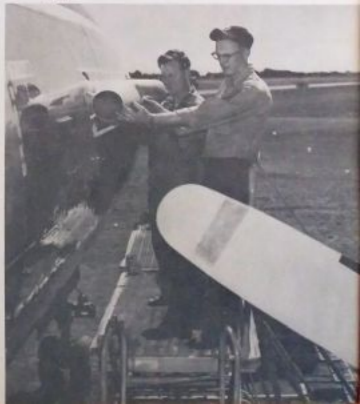
New Zealand National Airlines Corporation mechanic and Kenneth A. Kellett, AE1, install insect trap on R7V.
