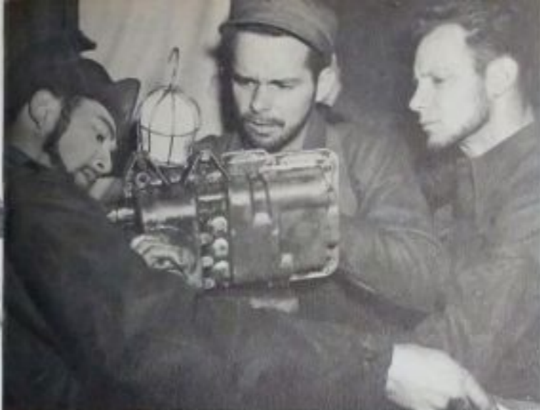
Fred S. Crumbliss, CMA3; Jerry E. Butler, CMH2, and David E. Williams, EOC, repair the clutch from a disabled snow cat.
